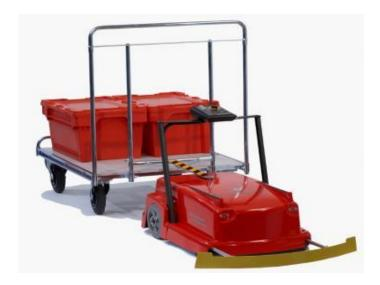
The Autotruck - suitable and designed for internal, light material handling applications, and is an alternative to trolleys and towing trucks.
