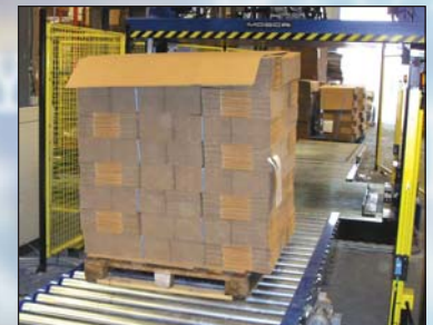
Pallet Conveyor incorporating Strappers
