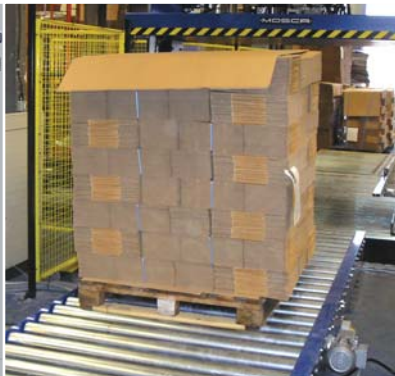
Pallet Conveyor incorporating Strappers
